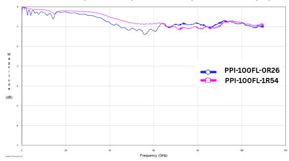
Inductors are mounted in two-port shunt configuration on 10 mil Rogers 4350B. Mounting angle is 45 degrees.
