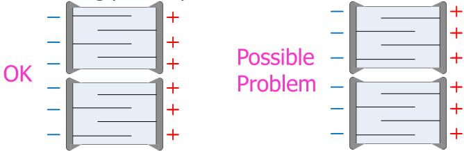
Voltage arc-over because of proximity to circuit board
