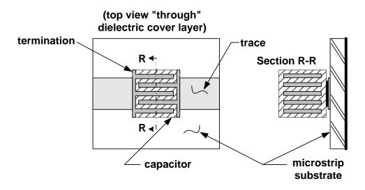
Features: (1) A ceramic brick with interleaved metallic electrodes
