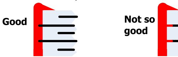
Design inadequacy: Outer electrode edge under termination overlap (drape)
