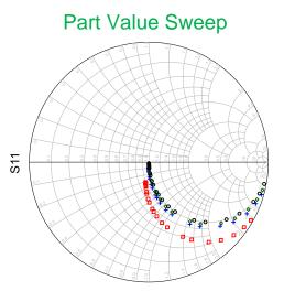
Legend:  $\Box$  4 mil Rogers 4350B, + 20 mil Rogers 4003C,  $\Diamond$  60 mil Rogers 4003C,  $\Diamond$  1deal Model S11 at 0.3 GHz for capacitor values from 1.0 to 470 pF on various substrates compared to an ideal capacitor response.
