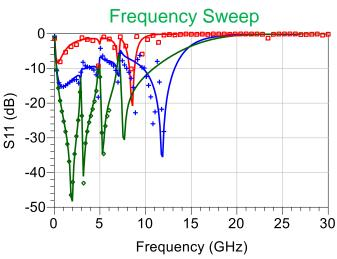
Legend: 4 mil Rogers 4350B, + 20 mil Rogers 4003C,  $\Diamond$  60 mil Rogers 4003C, Lines - Model, Symbols - Measured data. Measured data stops at highest valid frequency for each substrate. S11 for a 20 pF capacitor mounted on various substrates from 0.05 to 30 GHz.
