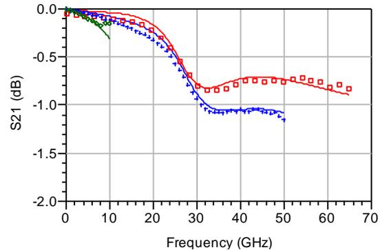
egend: □ 4mil Rogers 4350B, + 5mil Alumina, ◇ 31mil Rogers 5880, Lines - Model, Symbols - Measured data. Measured data stops at highest valid frequency for each substrate.
